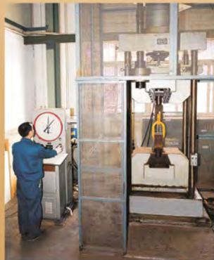
Tensile Test, Capacity 100 tonnes
