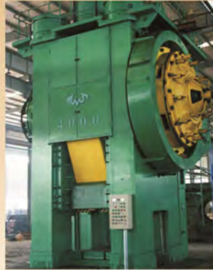
Forging Press 4000 Ton capacity
