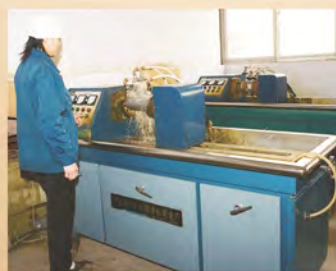
Magnaflux Crack Detection
