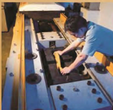
Tensile Test, Capacity 200 tonnes
